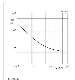
Fig.4 Differential forward resistance as a function of forward current; typical values.
